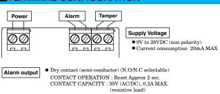
CONTACT CAPACITY: 30V (AC/DC), 0.1A MAX.
